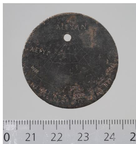
Figure 4. Disk showing the horary drawing for the latitude of Alexandria. One can clearly see that the hole is displaced relative to the drawing and that the latter is quite crude. Below the lines are the names of the months.
